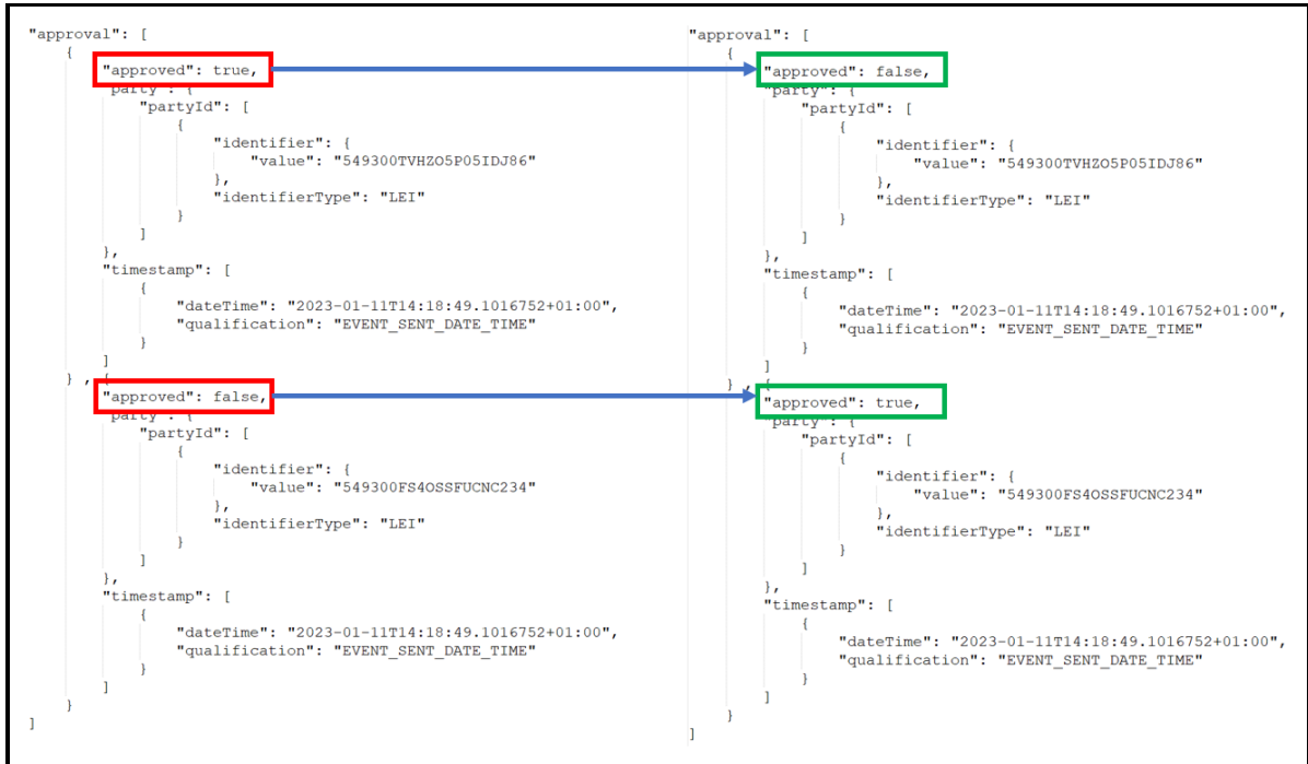
Diagram 26: The borrower (LEI “549300TVHZO5P05IDJ86”) sent the initial “approval” object through with their status set to “true” and the lender’s status (LEI “549300FS4OSSFUCNC234”) set to “false”. In the counter proposal the lender must set their approval status to “true” and the borrower’s approval status to “false”.
